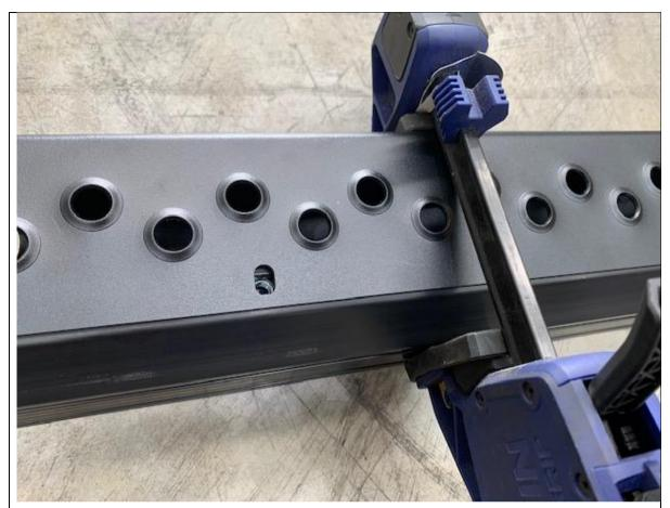
44. Using long tool feed nuts in to centre first and thread in with black M8 button head cap screws and washers.
