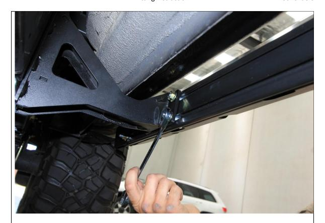
58. Tighten all mount to slider M10 flange nuts using 15mm spanner. A ratcheting spanner makes this process easier .
