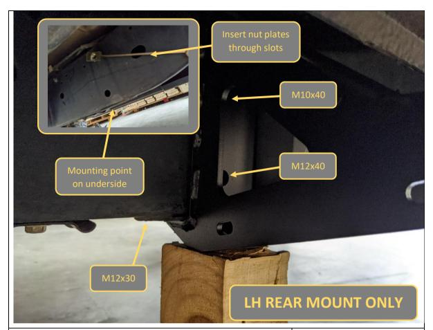
26. Offer up rear mount to mounting location, hold mount in place using jack and wood block to make positioning the nut plates easier.
