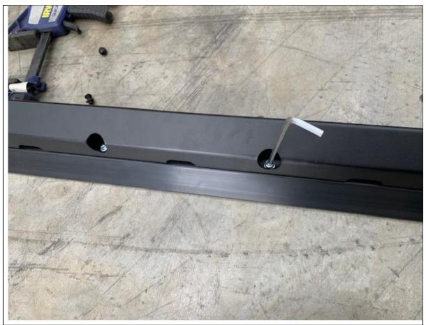
41. Thread cap screws into each hole
