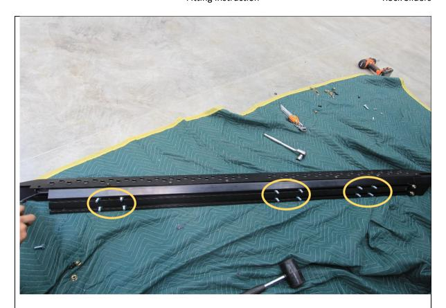
49. Slide the 12x M10x25 Hex bolts into the T slots on back side of extrusion. 6 bolts per slot.
