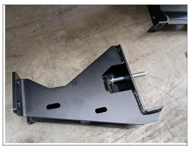
16. Prepare mid mounts by pre-inserting the M12x90 Bolt, with flat washer, part way through the top mounting hole.
